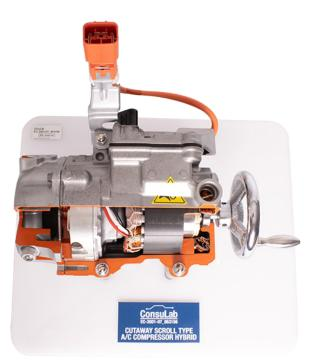
The ConsuLab EC-2001-07\_053156 is a complete scroll-type AC compressor from a modern hybrid vehicle with included 3-phase electric motor. The compressor and motor are cutaway to allow students to see internal operation. The unit can be rotated by a hand crank. Includes the orange high voltage wiring connector and wiring loom.
