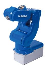
The MotoMini robot is the smallest and lightest 6-axis robot in the industry. The 7-kg (15.5 lb) robot is easy to carry, ship and install.
